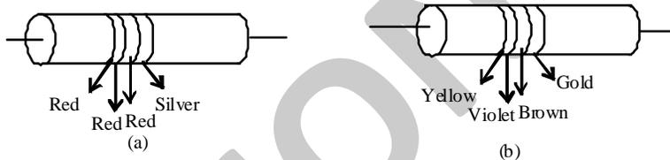
**Illustration 11.** The figure shows a colour-coded resistor. What is the resistance of this resistor?
